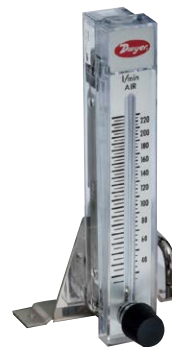
Calibrated flow meter Cat.No. 710-0965
